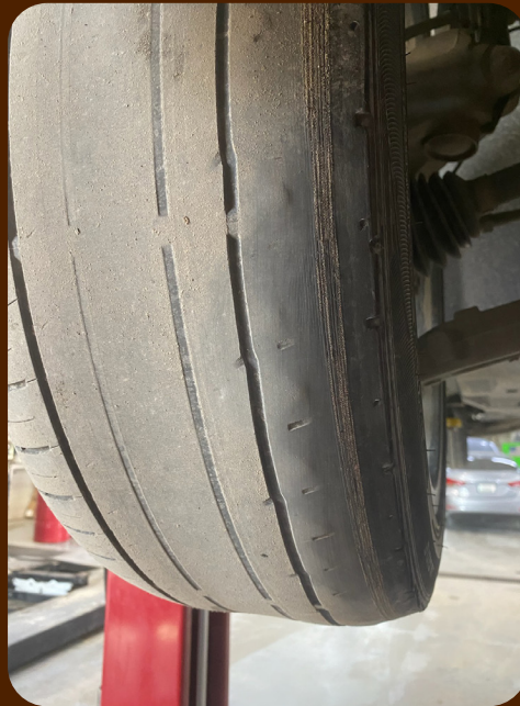
Missouri safety inspection found a driver had driven this defective tire until the tire tread was completely gone.
