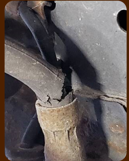
Missouri safety inspection located this defective brake hose.
