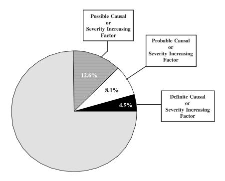
Note: In total, 25.2% of the 420 traffic crashes studied had a definite, probable, or possible vehicle defect that contributed to the cause of the crash or increased its severity.
