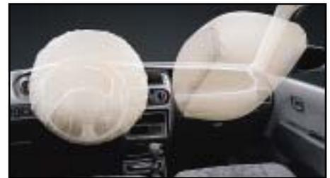
is often coated with starch or talcum powder to prevent its neoprene lining from sticking together while in storage. The passenger side bag is rectangular, emerges out of the dash, and is not packed with starch. With this in mind, the Trace
