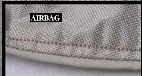
*Vent holes are designed in the airbag to allow hot nitrogen gas to escape. However, hot gas can also vent through the seams in the front of the airbag. If clothing comes into contact with a maximum inflated airbag, the hot gas can cause single patterns characteristic of the seam patterns, which appear as a series of small dots or smears. Stitching patterns can vary from one airbag to another, by make, model, and year, thereby yielding class characteristics.*
