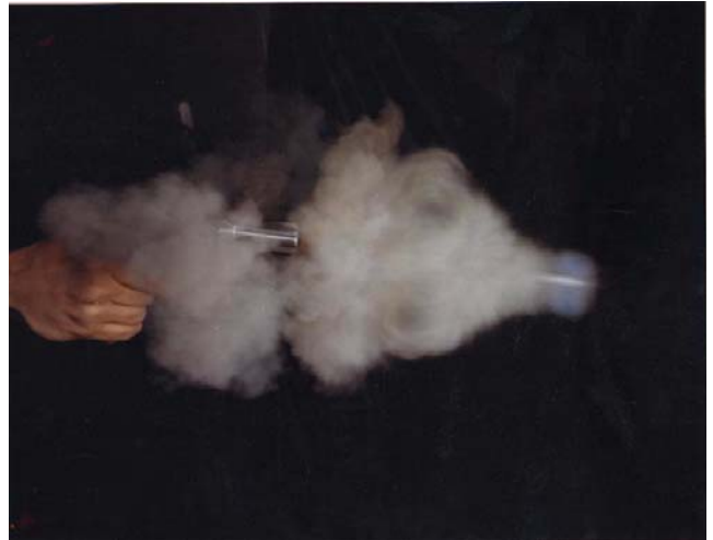
A vaporous cloud of smoke containing microscopic GSR particles is discharged upon firing a gun. This high speed photograph demonstrates how GSR particles (in the white cloud) can be deposited onto surrounding surfaces, especially the hands.
