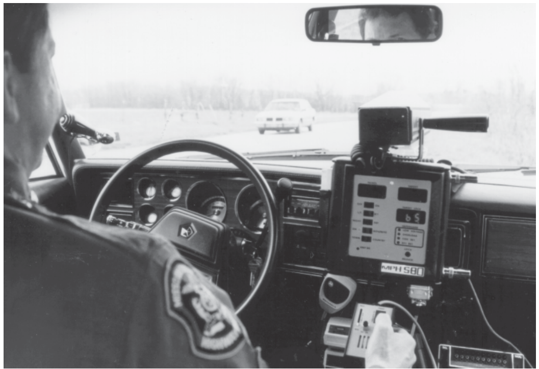
A trooper uses the new 600 MPH S-80 MCX radar unit.
