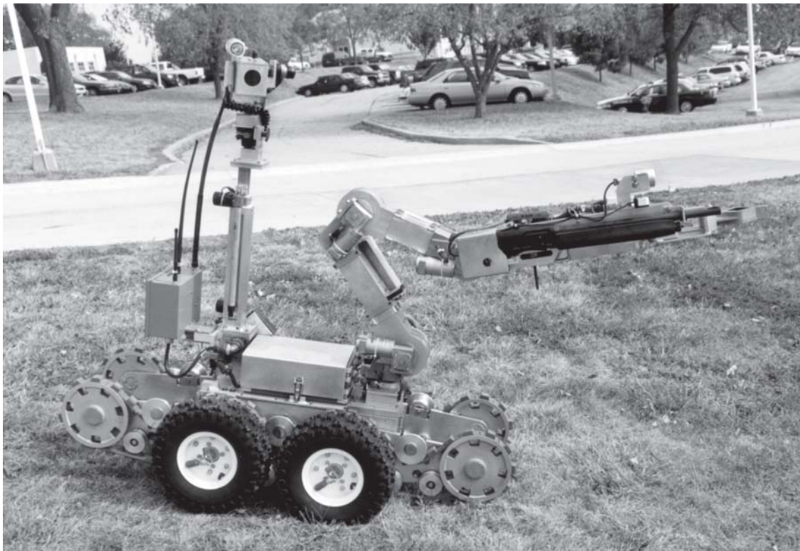
This Romotec F6A robot allows technicians to render bombs safe from a distance.
